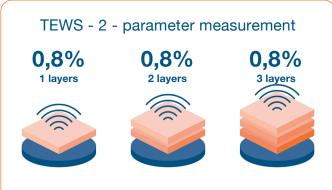
3 layers of the same material show the same moisture, the density is recognized and moisture results compensated  $\rightarrow$  correct results
